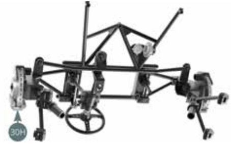
Preassembly of front suspension and steering
