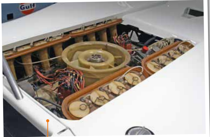
The impressive cooling turbine covers the flat 16-cylinder, surrounded by bulky detonators.
